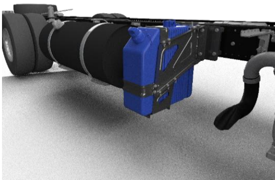
BS 6 chassis are equipped with an "AdBlue®" tank
